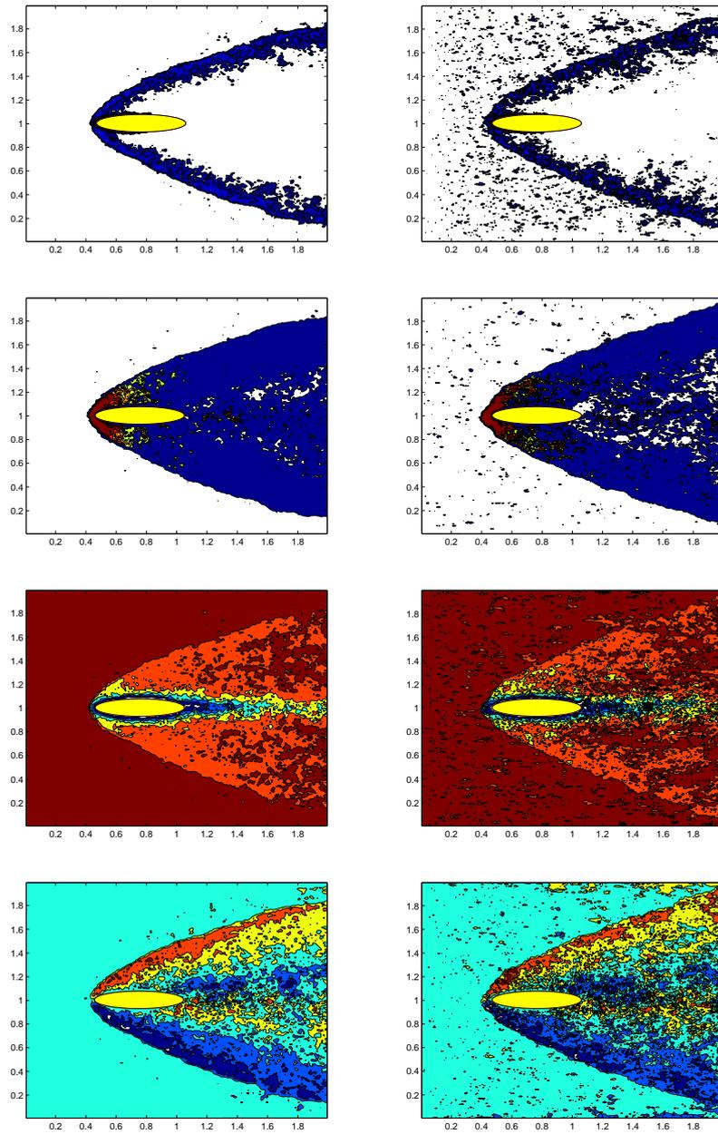
**Fig. 1.** 2D flow: Domain Decomposition Hybrid scheme(left) Monte Carlo (right) density (top), temperature (middle) velocity x- direction (middle) and velocity y- direction (bottom)
